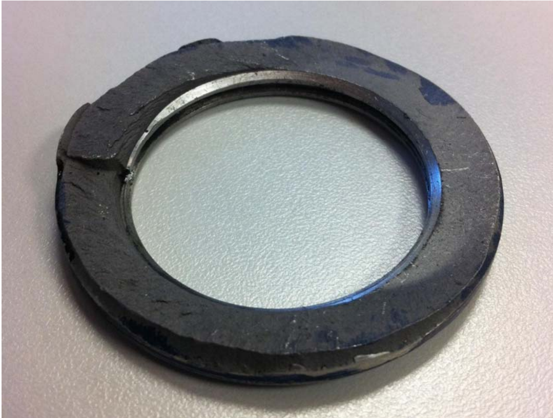
Ring of failure point on -91 titanium socket (Test #1), failed at 104k cycles
