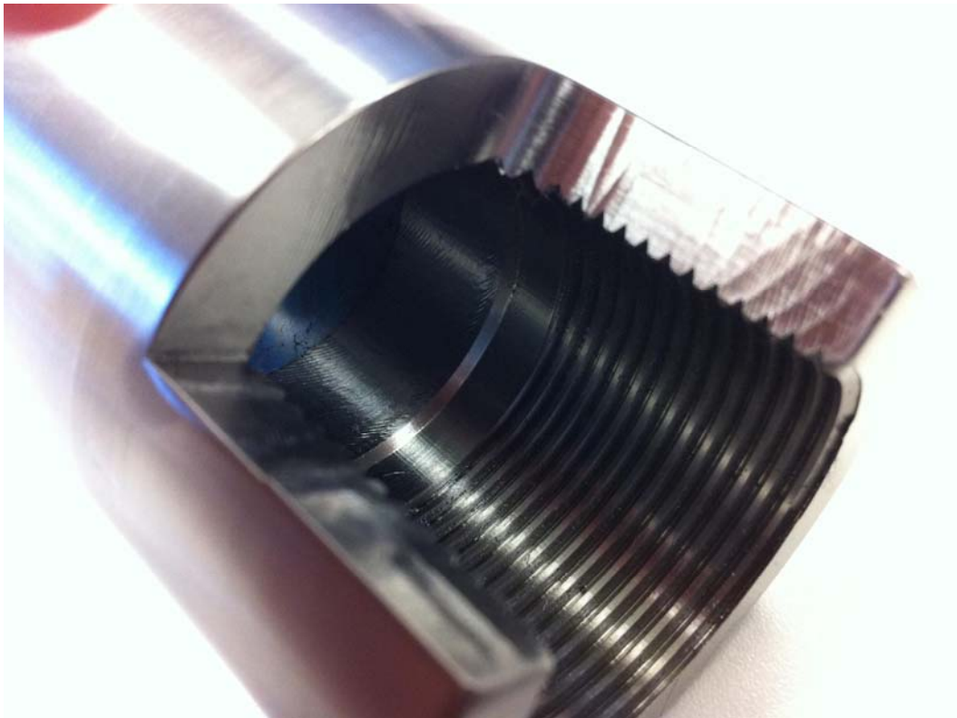
Photo of inside intact socket from opposite end of Test #2 sample, went 96k cycles
