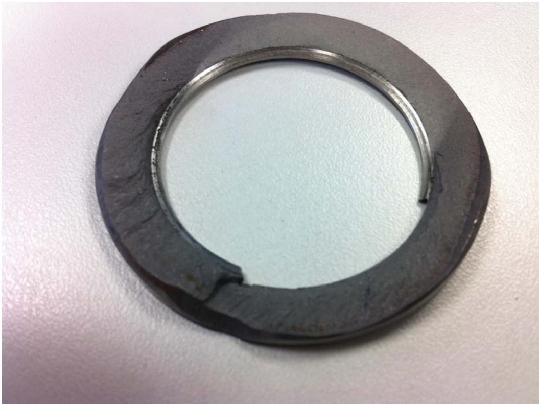
Ring of failure point on -91 titanium socket (Test #2), failed at 96k cycles
