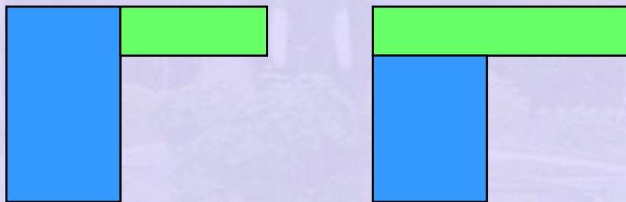
Figure 9-3.13 Component rectangles of a compound section
