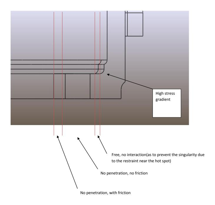
I splitted the inner hub flange, to make the restraint "softer" to be able to get some sort of convergence.
