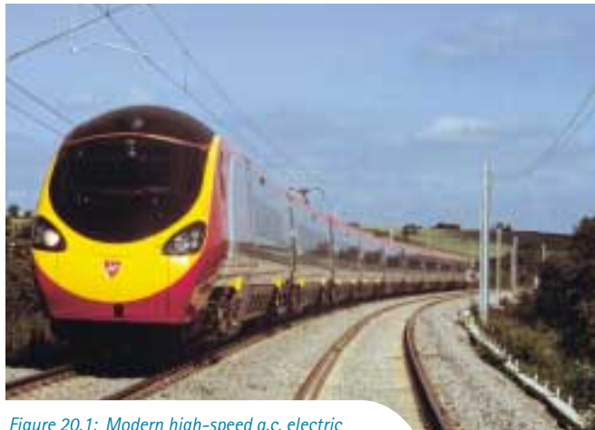
Figure 20.1: Modern high-speed a.c. electric inter-urban train
