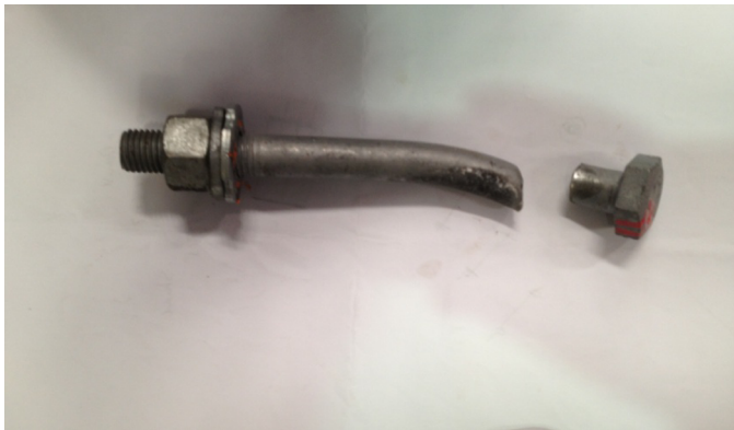
Fig. 10. Shear fracture failure of bolt in specimen SP3
