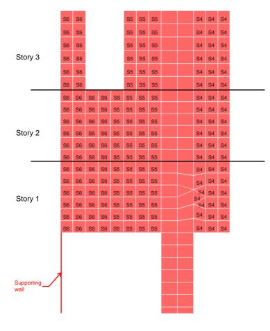
To monitor positive moment at mid of the wall, wall is assigned into to labels in the first span ..
