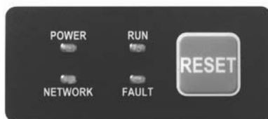
Figure 6 LED Status Indication and Reset
