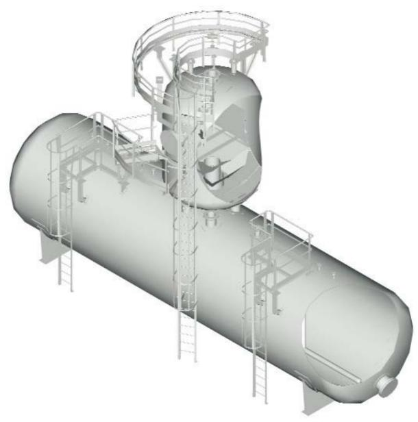
The thermophysical deaerator is by far the most applied technology when oxygen and carbon dioxide in Boiler Feed Water must be reduced to negligible concentrations
