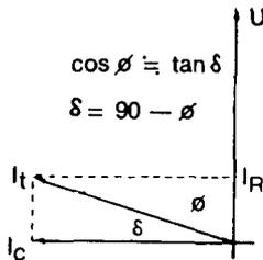
Fig. 2.3 Vector diagram to represent dielectric loss angle
