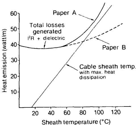
Fig. 2.11 Thermal stability of a buried 2000 mm<sup>2</sup>, 400 kV cable with a current of 1400 A
