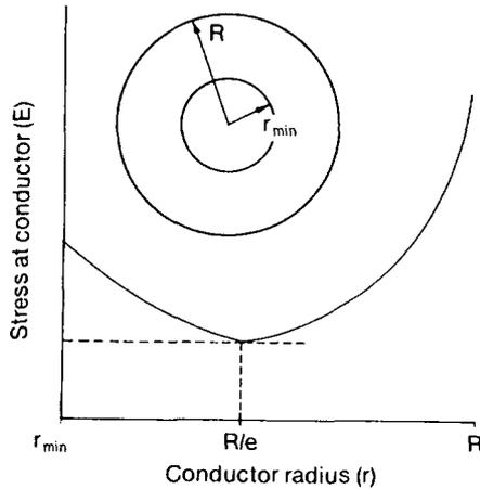
**Fig. 2.6** Variation of stress with conductor radius
