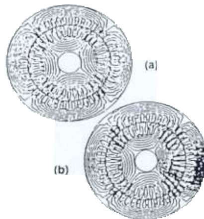
Fig. 6 - The field distribution at full load (1760 rpm). (a) no broken bars (b) five broken bars
