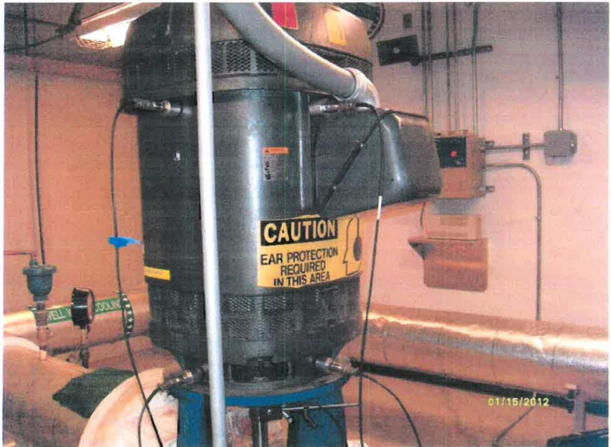
WP 1 VIBRATION SET UP VERTICAL (Y) INLINE WITH PIPING HORIZONTAL (X) PERPENDICULAR TO PIPING
