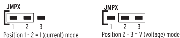
Figure 2.3 Circuit Board of Analog I/O Board, Showing Jumper Selection
