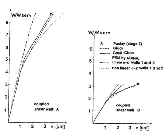
Fig.4 Comparison of the continuous methods and the FEM
