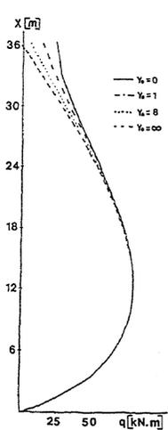
Fig.5 Top stiffening beam's design: laminar shear force
