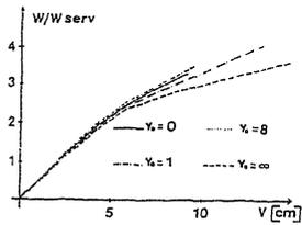
Fig.6 Top stiffening beam's design: structural and rotational ductility
