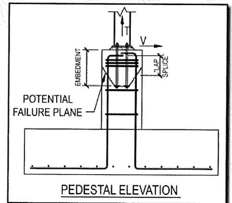
If the shear and/or tension forces on the anchor rods are small or the footing is large, the Appendix D provisions can easily be met. With moderate to large shear and/or tension forces on the anchor rods or base plates near edges, the provisions of Appendix
