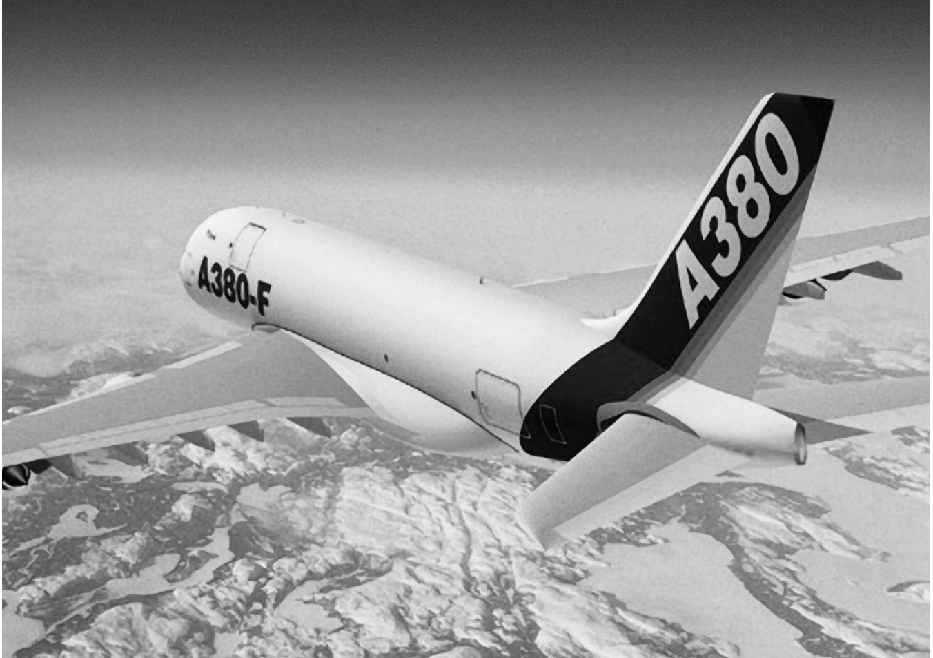
A380 Airbus Using GLARE Laminate with S-2 Glass Yarns for Aircraft Skins, Floor Panels and Fire Walls
