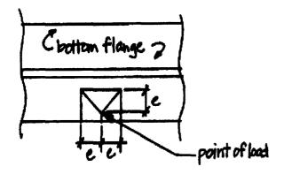
The section modulus at the plane of bending is  $(bd^2)/6$  which translates to  $e(t_f)^2/3$ . From Figure 2 the bending moment is eP/4. The bending stress is:
