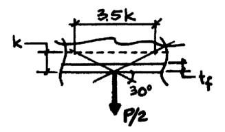
Flange bending depends on the location of the wheels with respect to the beam web. Referring to Figure 2, this is dimension e. As stated previously, each wheel load is P/4.
