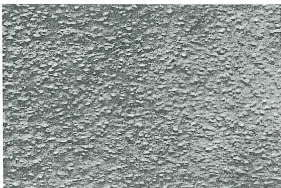
FIG. D Abrasive Floor or Tread Plate Rolled in both steel and aluminum
