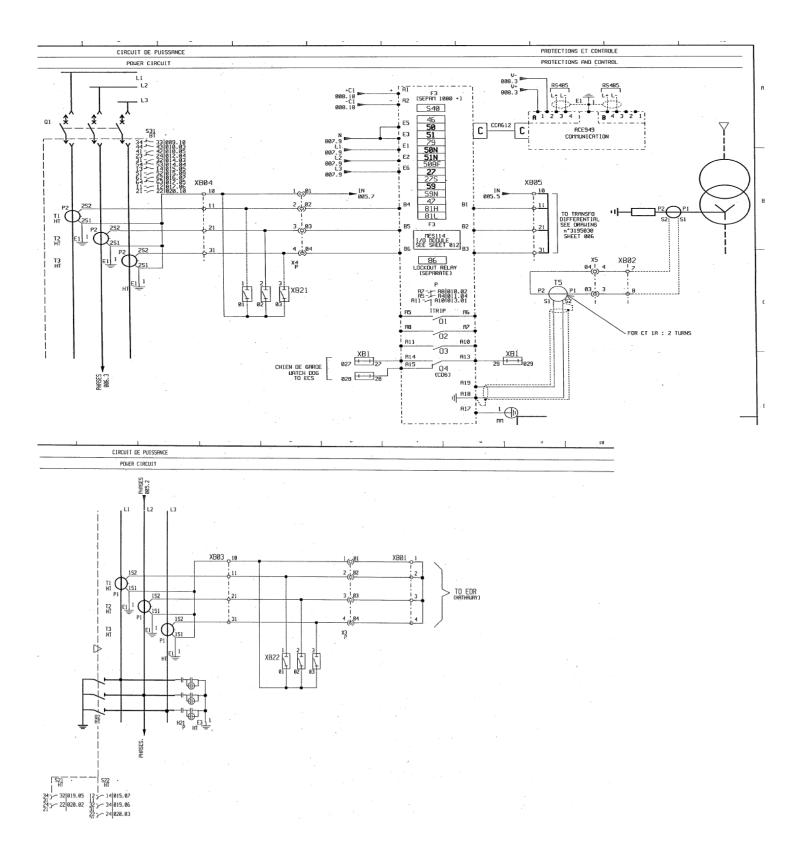
INCOMER POWER CIRCUIT DIG. IT KEPT ON WORKING AND ITS SEPAM REGISTERED "BLOCKING TRANS".
