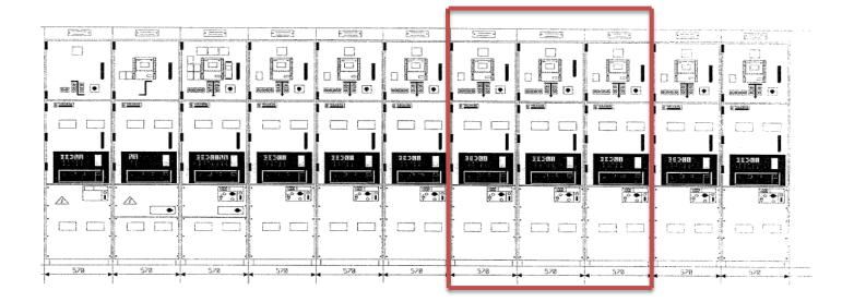
FEEDERS HAVING SAME CT RATIO 50/1 AND SAME EARTH FAULT SETTING WERE TRIPPED.
