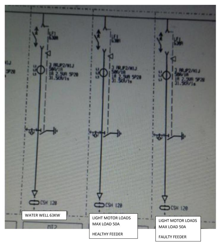
SINGLE LINE DIAGRAM OF THE FAULTY FEEDER AND TWO ADJACENT FEEDERS. ALL TRIPPED ON EARTH FAULT.
