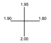
5. Radial clearance (with lead wire) of main bearing: 0.35 mm
