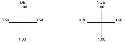
4. Air Gap between Exciter Stator & Rotor (in mm):
