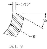
NOTE 1 - Pre-fabricated half sole to extend 1/2 inch past center on both sides for both top and bottom half soles to allow field installer to trim to fit. Installer will trim and bevel edges per Detail 3.
