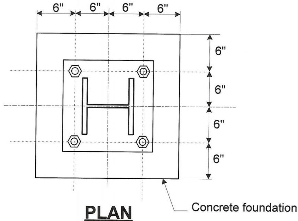
**Supports for Constant Support Springs at Wellhead Flowlines**
