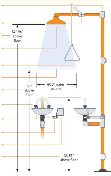
Location: Install safety station within 10 seconds (approximately 55 feet) of hazard, on the same level as hazard and with unobstructed travel path. Where strong acids or caustics are being handled, safety station should be located adjacent to the hazard, and an appropriate professional should be consulted for advice on the proper distance. (Section 7.4.2; B5)
