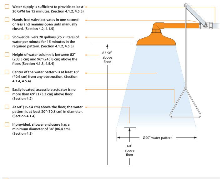
**Location:** Install shower within 10 seconds (approximately 55 feet) of hazard, on the same level as hazard and with unobstructed travel path. Where strong acids or caustics are being handled, emergency showers should be located adjacent to the hazard, and an appropriate professional should be consulted for advice on the proper distance. (Section 4.5.2; B5)
