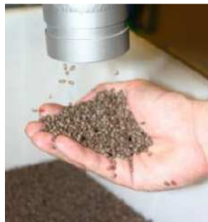
Fig 13 Extruded natural fiber and thermoplastic resin beads
