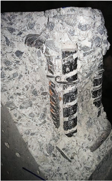
Figure 9 Signs of slippage in basalt reinforced beams
