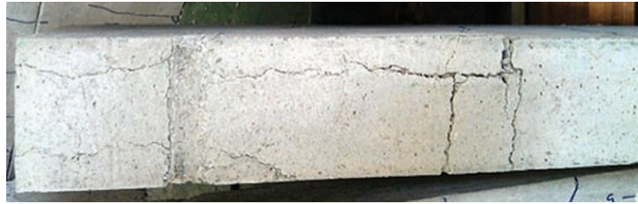
Figure 10 Crack propagation on underside – spanning length of beam
