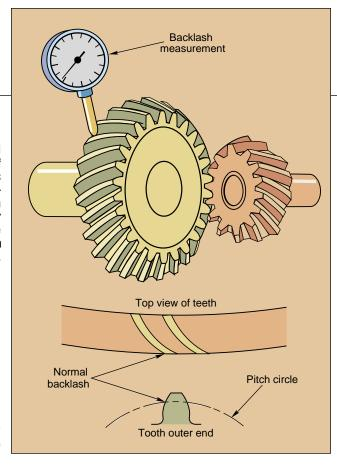
Figure 3 — Normal backlash in a set of spiral bevel gears is measured perpendicular to the tooth surface at the outer end (heel) of the tooth, using a dial gage.
