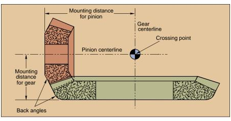
Figure 1 — Mounting distances used for assembling bevel gears.
