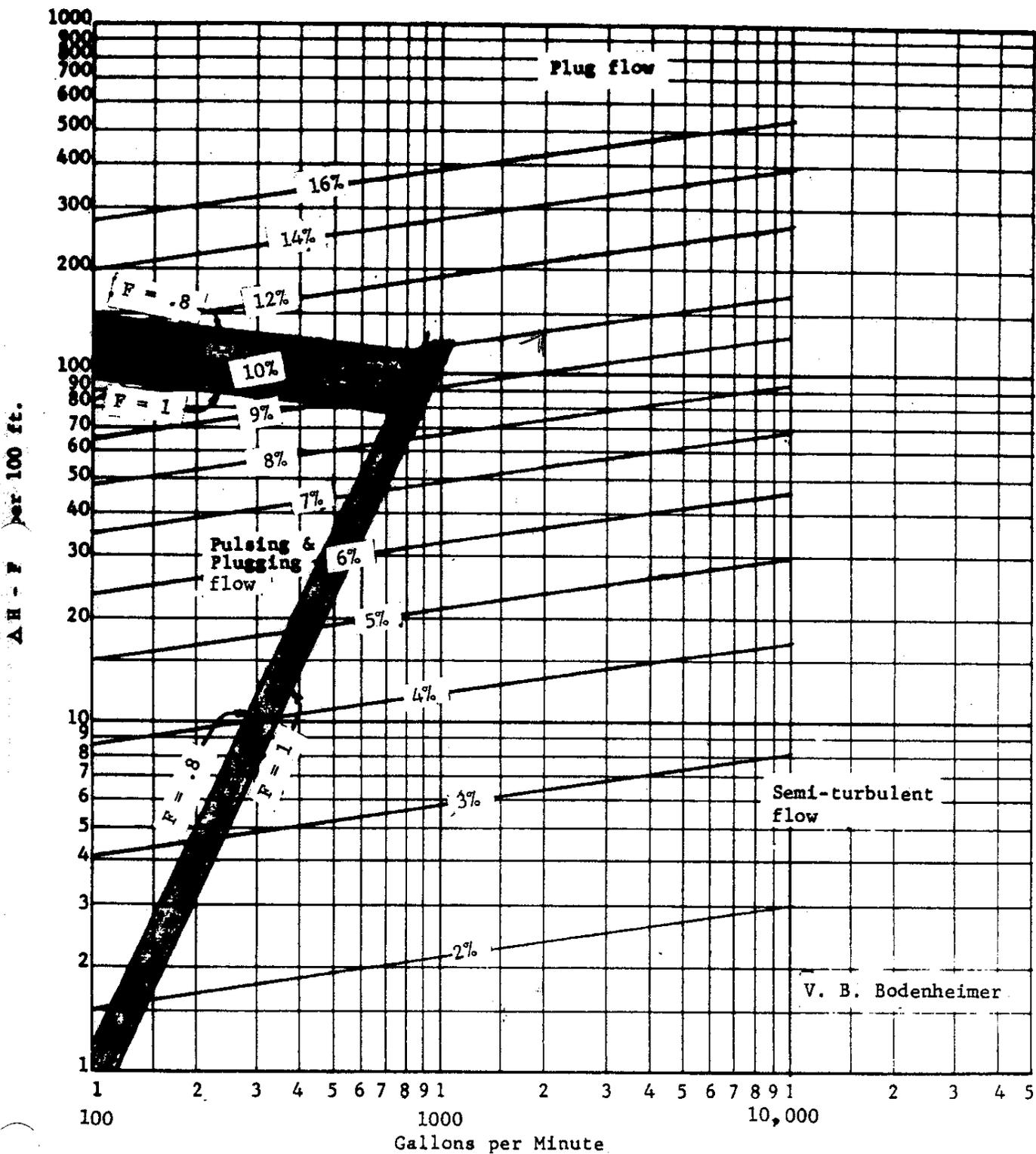
FRICITION LOSS IN 19.72" I. D. STAINLESS STEEL PIPE
