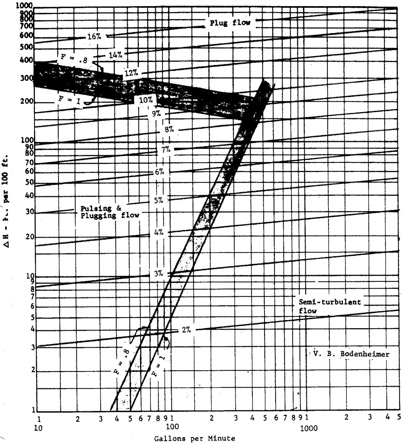
FRICITION LOSS IN 10.532" I. D. STAINLESS STEEL PIPE
