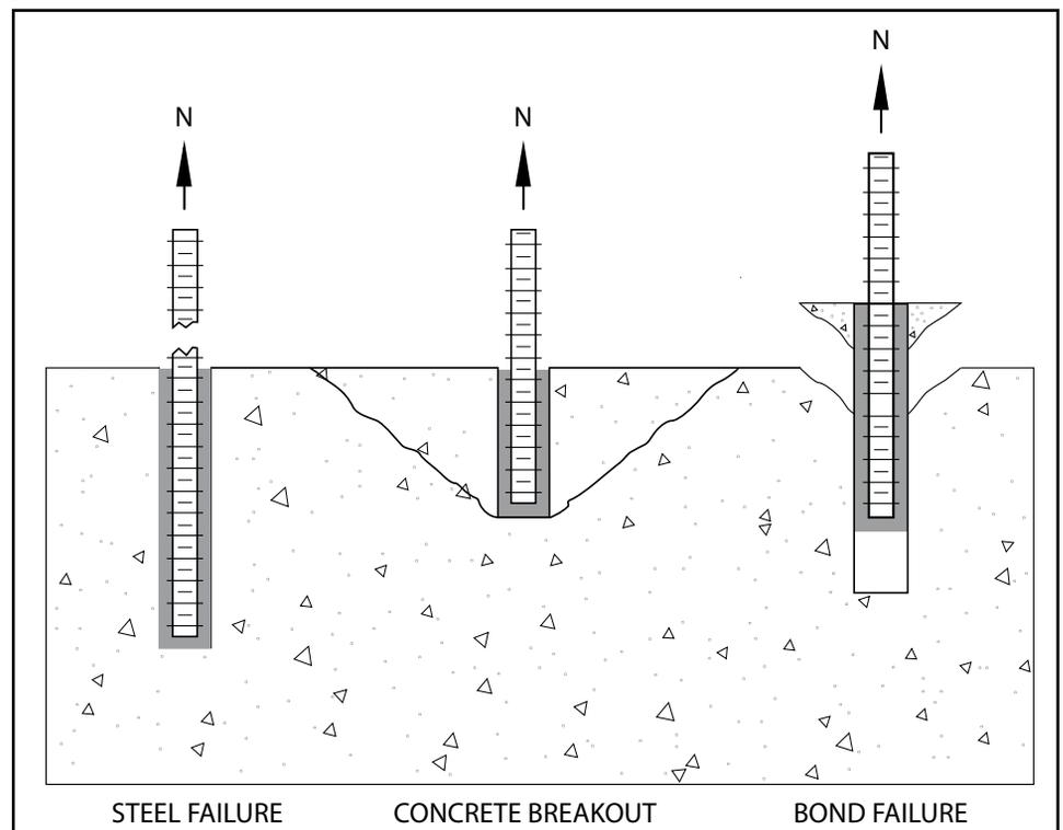
Figure 1: Failure modes for adhesive anchors.
