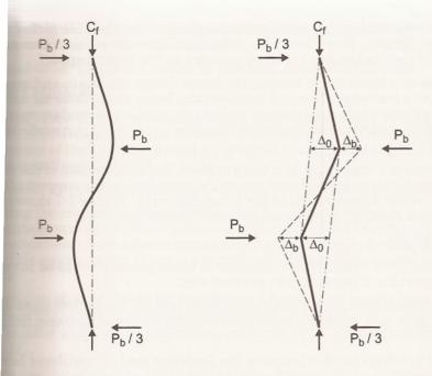
The solid line represents the initial misalignment. The dotted line represents the final displaced configuration due to all the forces acting on the system.
