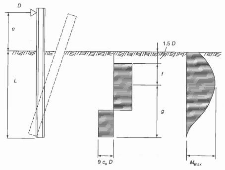
**FIGURE 8.2**Deflection, soil reaction, and bending moment distributions for laterally loaded short piles in cohesive soil. (From Broms, B., 1964a, *J. Soil Mech. Found. Div., ASCE*, 90(SM3):27–56. With permission.)
