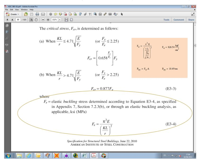
We can proceed as if assigning the case to a Dead load type in a on XZ **plane frame** analysis, except that the analysis will be for (elastic) buckling load.
