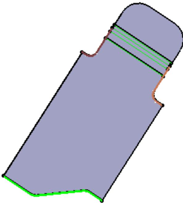
*Unfolded Surfacic Flange defined with Corners 1 and 2 of 10mm each, and no compensation for Side 1 and Side 2*
