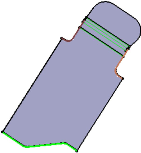
*Unfolded Surfacic Flange defined with Corners 1 and 2 of 10mm each, a Manual: Angle compensation of -20deg for Side 1 and no compensation for Side 2*
