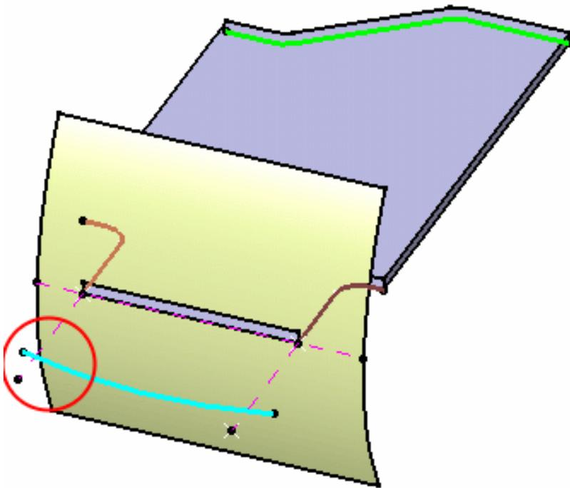
*There is an intersection between the OML and the EOP -> the Surfacic Flange can be computed*
