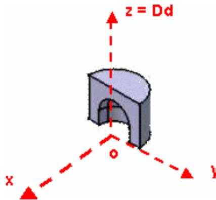
The die is applied matching  $Dd$  on  $Dw$  and matching the die's (x, y) plane onto the selected face:
