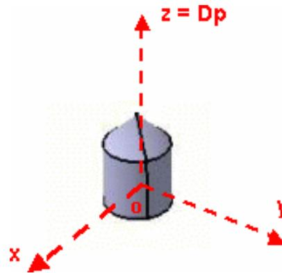
The punching direction on the base feature ( $Dw$ ) is normal to the selected base feature face, and is oriented from the selected base feature face towards the opposite face.
