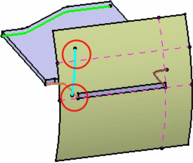
*There is an intersection between the side and the EOP but no intersection between the side and the OML -> the Surfacing Flange cannot be computed*
