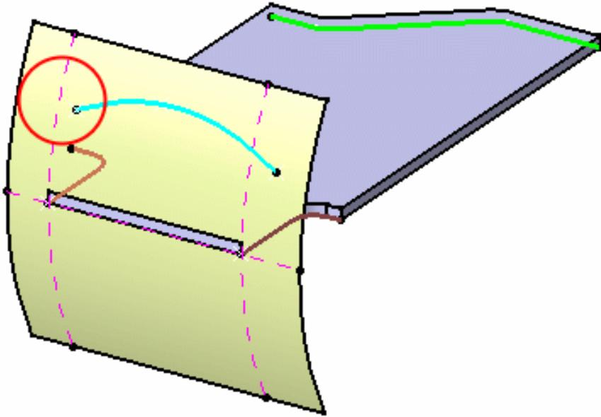
*There is no intersection between the EOP and the side -> the Surfacic Flange cannot be computed*
