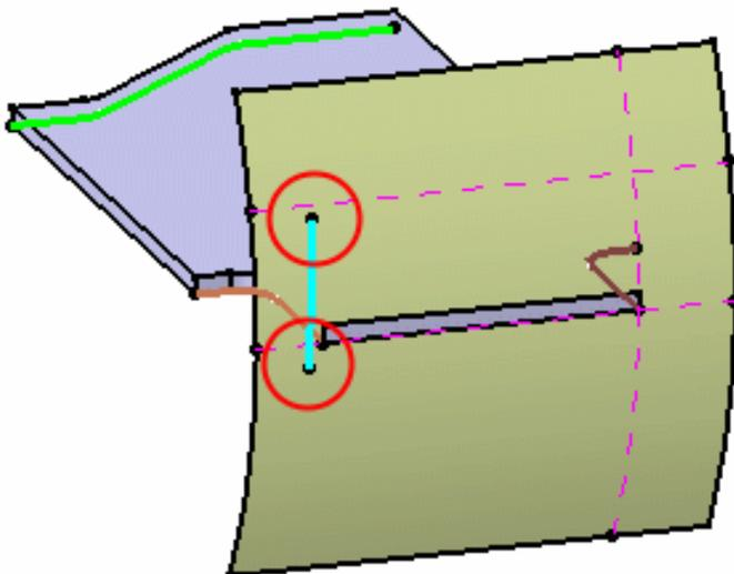
*There is an intersection between the side and the OML but no intersection between the side and the EOP -> the Surfacic Flange cannot be computed*
