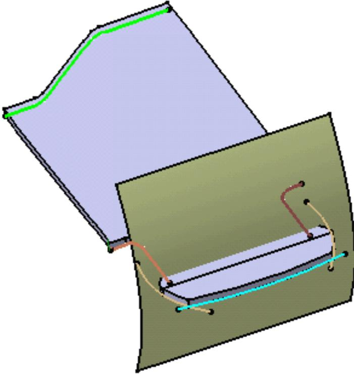
*Unfolded view of the Surface Flange with EOP FP as Element FP, Side 1 FP and Side 2 FP (in light brown) as Side 1 and Side 2.
