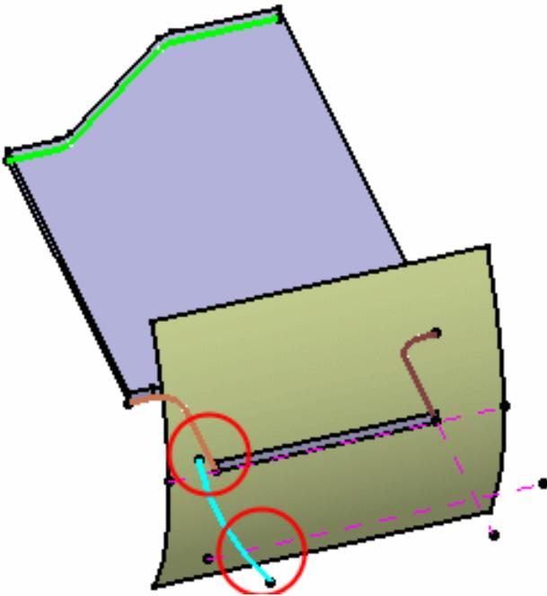
*There is an intersection between the side and the EOP and between the side and the OML -> the Surfacing Flange can be computed*
