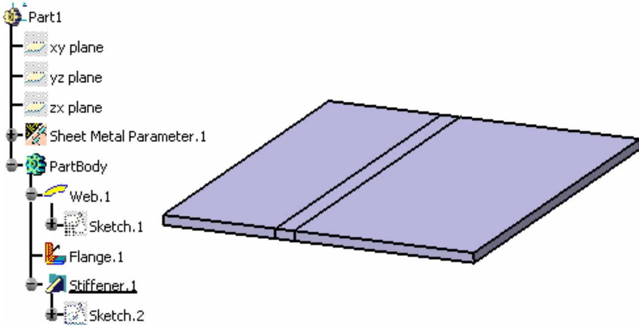
The stiffener is not displayed on the unfolded view.
