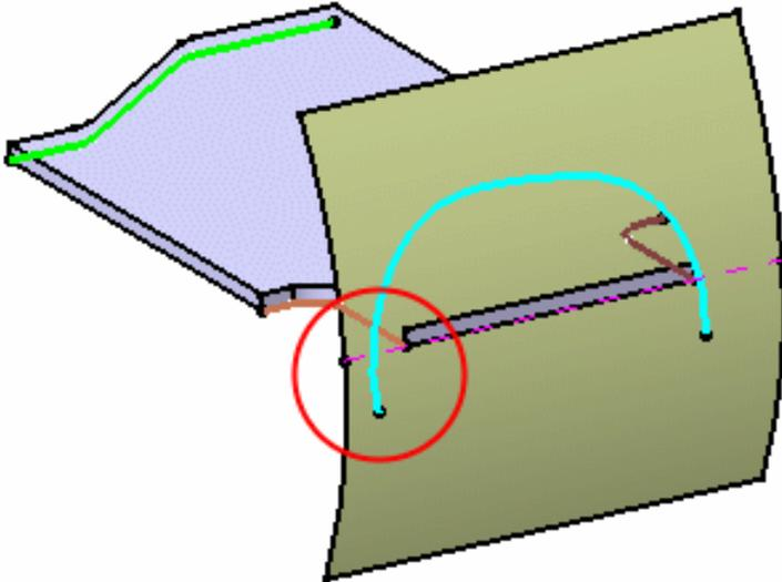
*There is an intersection between the EOP and the web support -> the Surface Flange can be computed*
