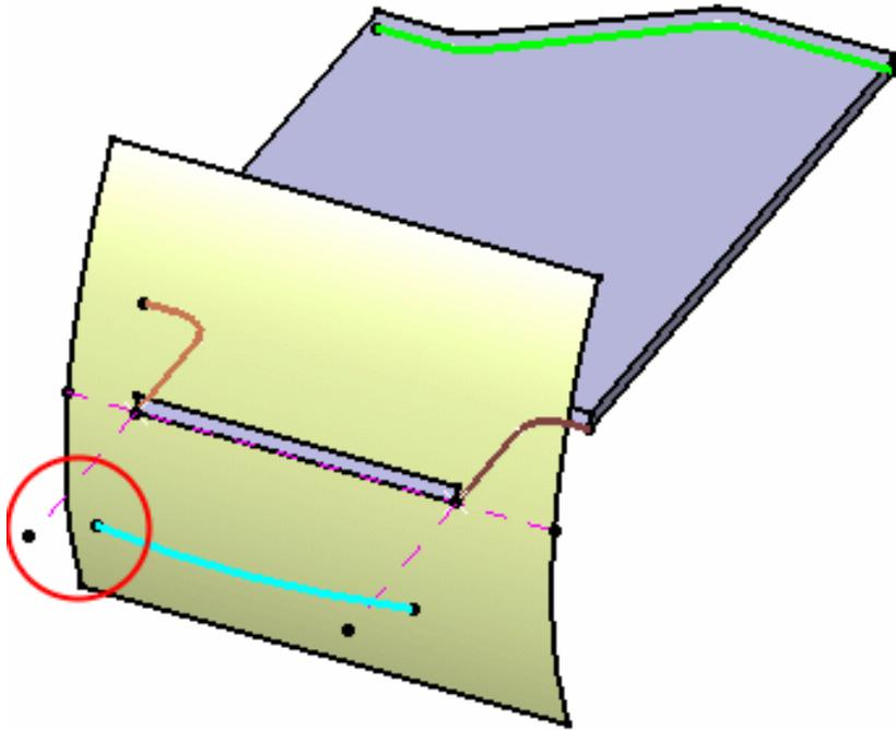
*There is no intersection between the OML and the EOP -> the Surfacic Flange cannot be computed*
