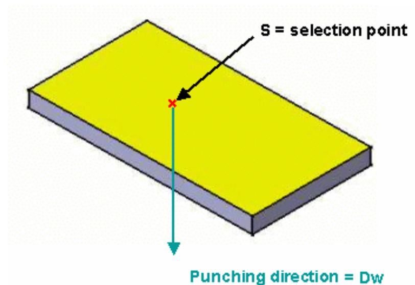
The punch is applied matching  $Dp$  on  $Dw$  and matching the punch's (x, y) plane onto the selected base feature face:
