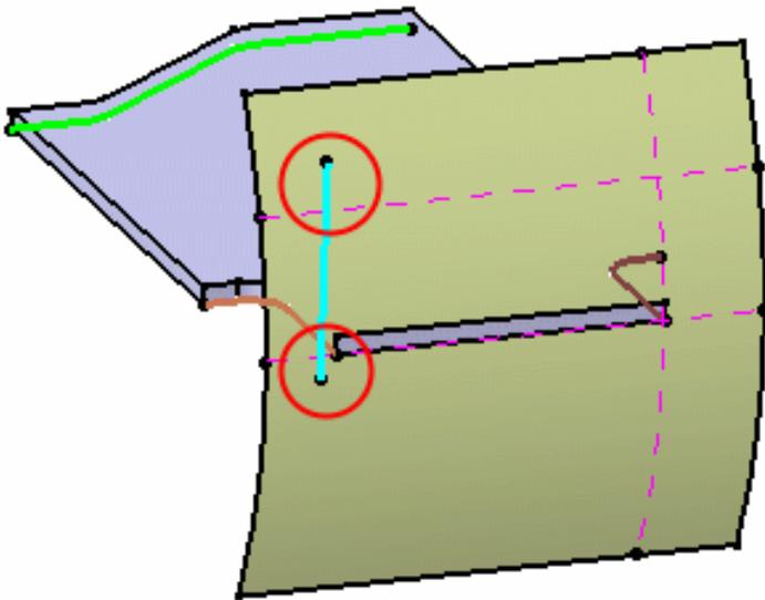
*There is an intersection between the Element FD and the OML and between the side and the EOP -> the Surfacic Flange can be computed*
