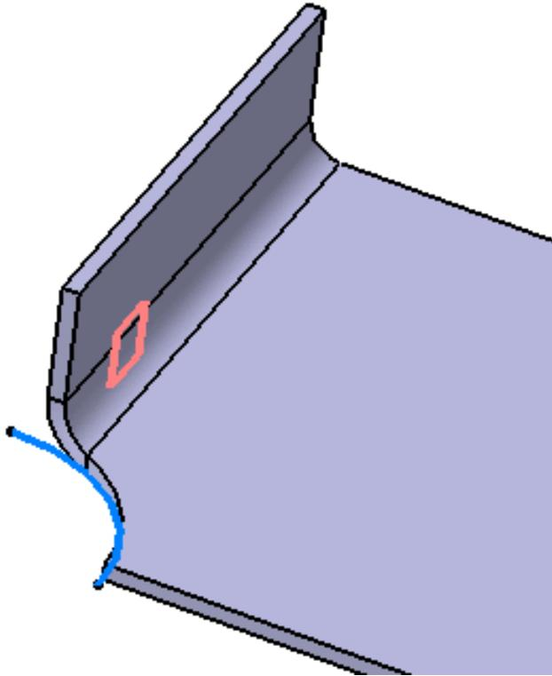
*The example above shows a Surfacic Flange with standard sides calculated from the web modified by a cutout (the cutout, shown in blue, is taken into account)*
