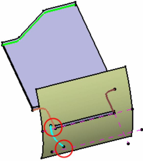
*There is an intersection between the side and the EOP but no intersection between the side and the OML -> the Surfacic Flange cannot be computed*
