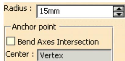
1. Define the default radius: it is equal to the bend radius + the thickness.
