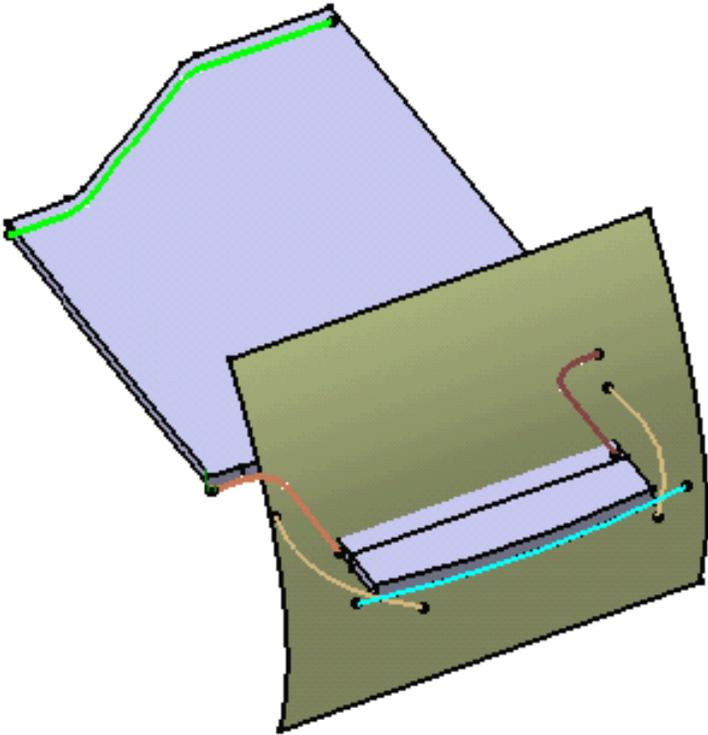
*Unfolded view of the Surfacic Flange with EOP FP as Element FP. See [Unfolding](#).*
