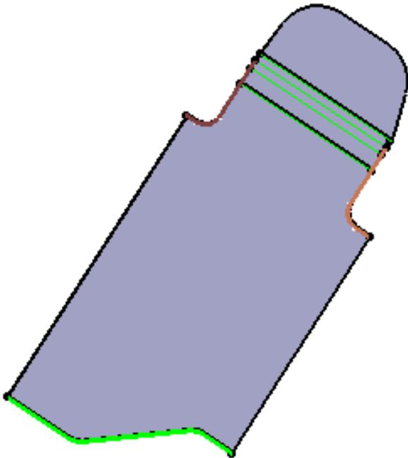
*Unfolded Surfacic Flange defined with Corners 1 and 2 of 10mm each, a Manual: Angle compensation of 20deg for Side 1 and -10deg for Side 2*
