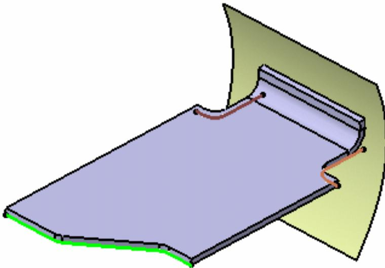
*Surfacic Flange with a length from OML of 15 mm*
