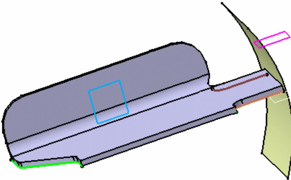
*The example above shows a Surfacic Flange defined with Sides 1 and 2 as Standard, and Corners 1 and 2 of 10mm each.*
