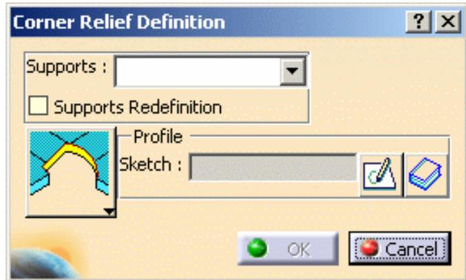
**2.** Select the supports on which a corner relief should be created (here we chose Surfacic Flange.1 and Surfacic Flange.2)
