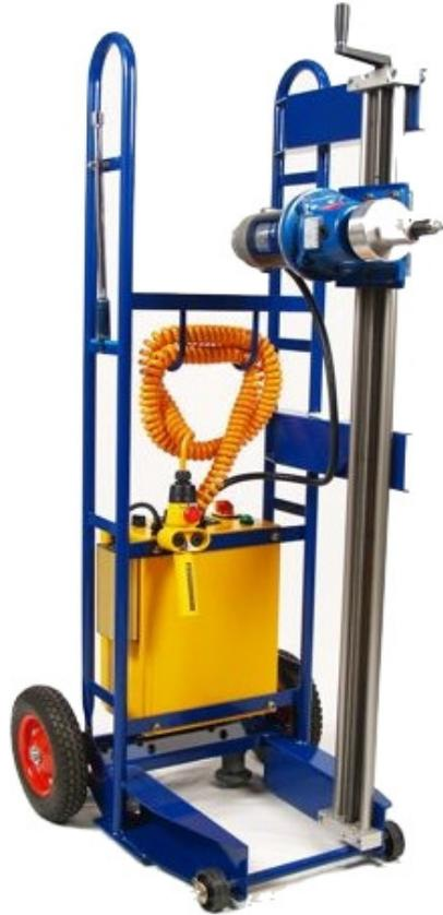
**CBS ArcSafe™** remote racking system enables service personnel to stand outside the arc flash protection boundary while racking low and medium voltage draw-out circuit breakers in or out. This eliminates the need for a full-body arc flash hazard suit.
