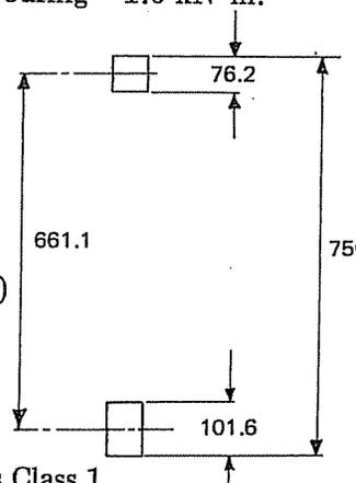
Note: top chord thickness is also governed by the requirement of shear stud welding.
