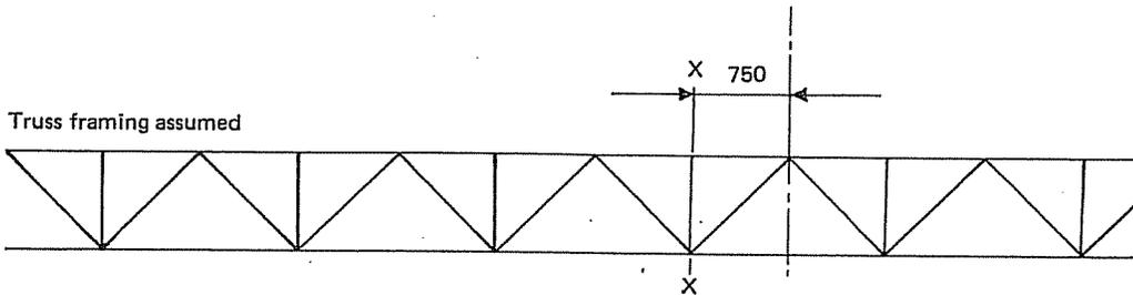
Assume factored bending moment on steel truss under slab pouring @ XX = 260 kN·m;
