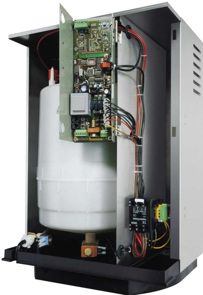
The steam humidifier Condair CP2 is a pressure-less steam generator designed for direct or indirect room humidification, using regular tap water or partially softened water.
