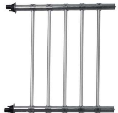
In combination with the Condair CP2, the multi-steam distribution system, OptiSorp makes very short humidification sections possible. The humidification distance is up to 4 times shorter than conventional steam distribution pipes.
