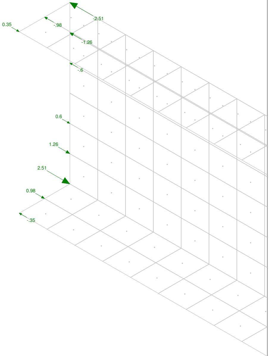
Loads: LC 1, Load at Shear Center
