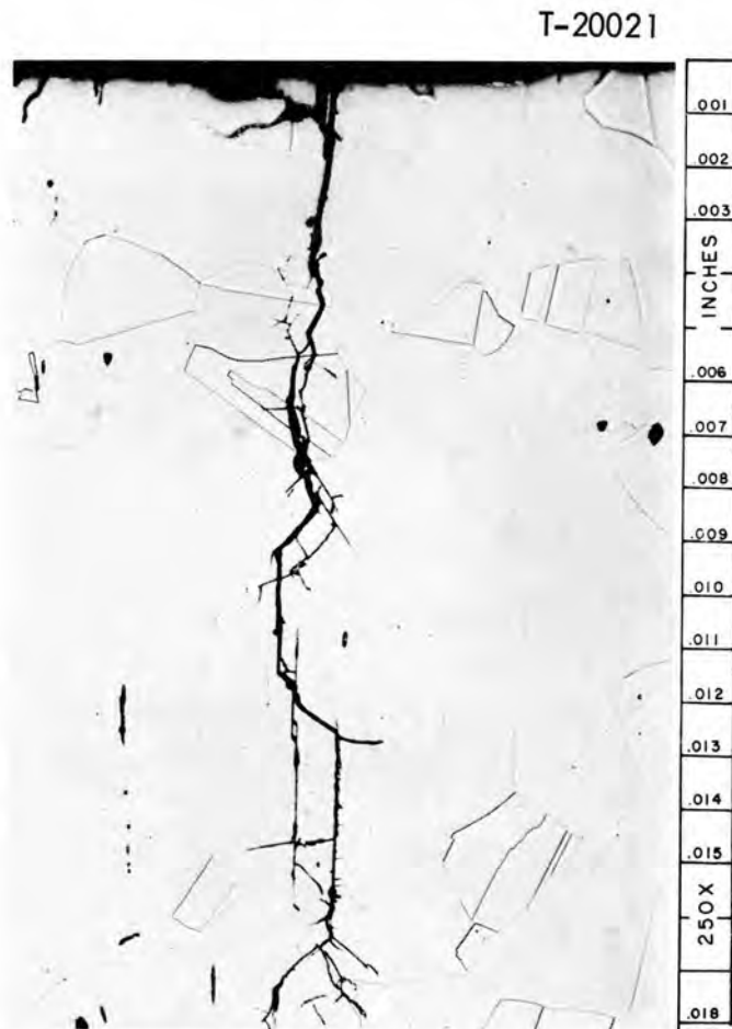
Fig. 31. Crack on ID of Type 304 Stainless Steel Pipe Specimen after 200 hr at 250°C in Water Containing 50 ppm Chloride, Etched in Glycemia Regia, X-250.
