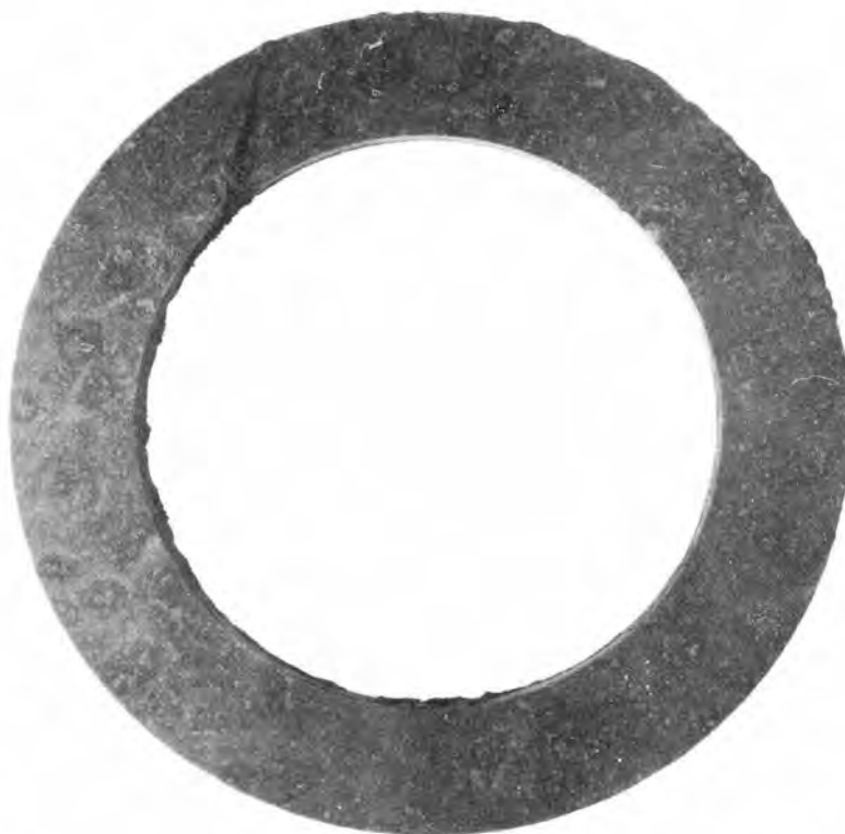
Fig. 27. Condition of Type 304 Stainless Steel Test Specimen after 100 hr at 250°C in Water Containing 100 ppm of Chloride, X-1.6.
