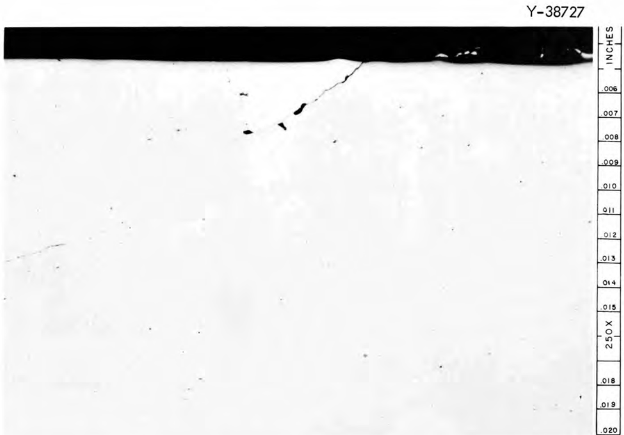
Fig. 22. Crack or Slag Inclusion in as-Received Pipe, as Polished, X-250.
