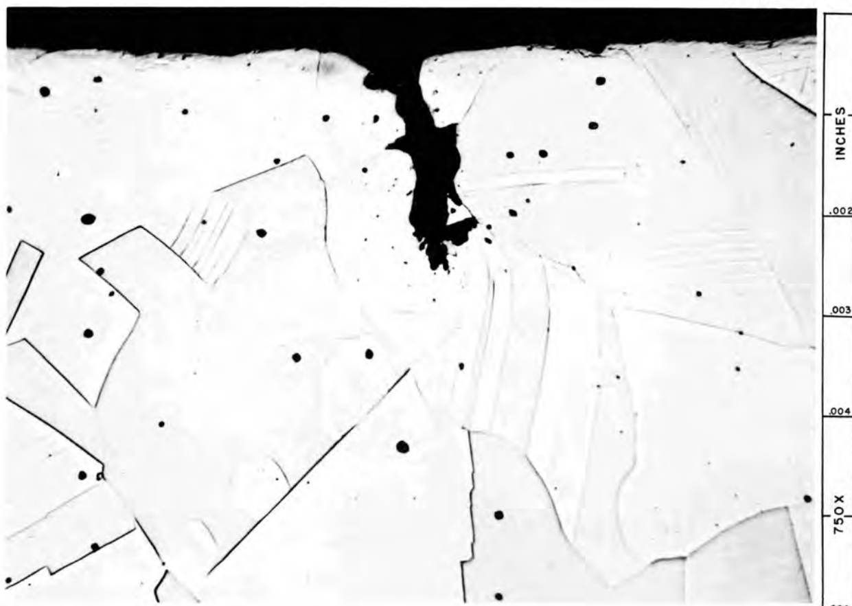
Fig. 14. Photomicrograph of Section 6, Fig. 8, Showing Penetration Normal to Surface, Etched with Modified Aqua Regia, X-750.
