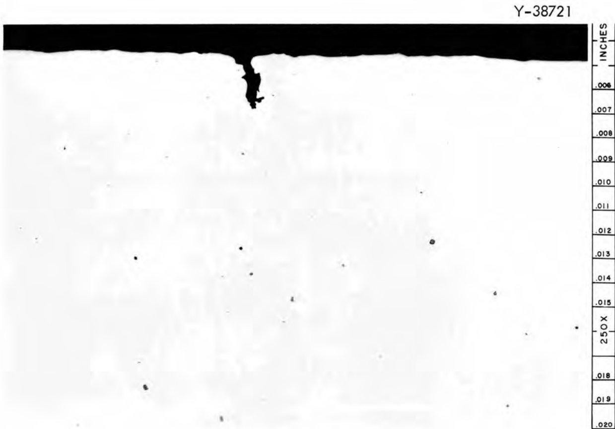
Fig. 12. Photomicrograph of Section 6, Fig. 8, Showing Penetration Normal to Surface, as Polished, X-250.
