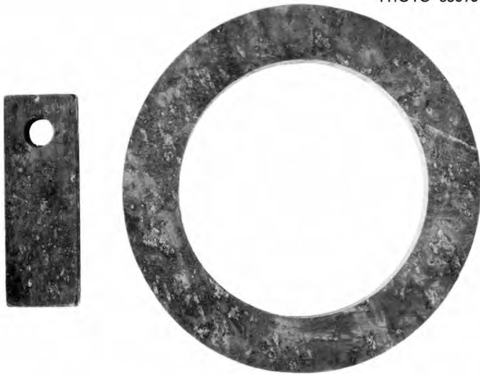
Fig. 28. Condition of Type 304 Stainless Steel Test Specimens after 200 hr at 250°C in Water Containing 50 ppm Chloride, X-1.6 (Test AN-40).
