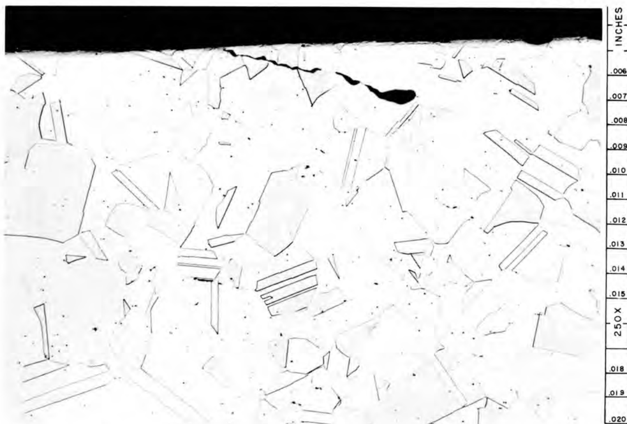
Fig. 25. Other Typical Defects in as-Received Pipe, Modified Aqua Regia Etch, X-250.
