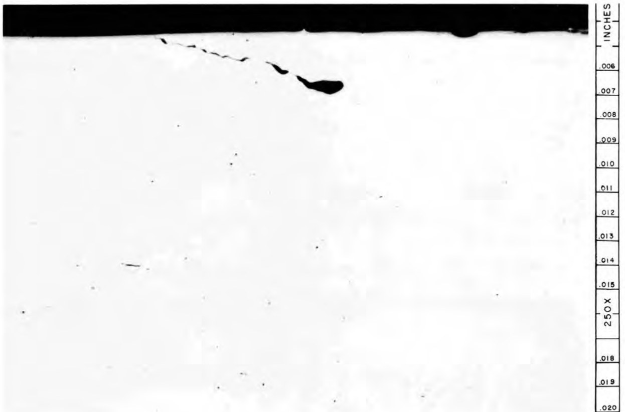
Fig. 24. Other Typical Defects in as-Received Pipe, as Polished, X-250.
