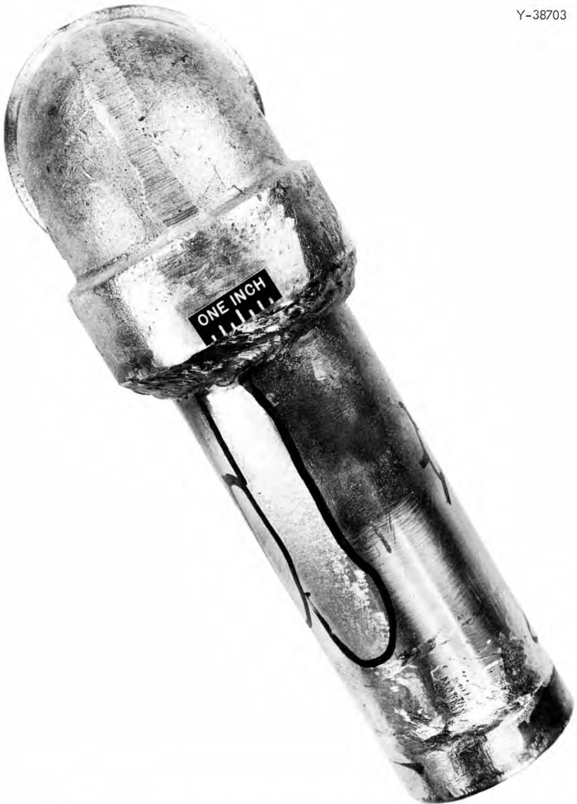
Fig. 2. In-Place Section of PP-1V Line after Cleaning at ORNL.
