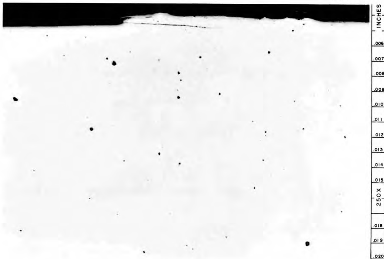
Fig. 20. Lap in Surface from Area Shown in Figs. 16 and 17, as Polished, X-250.
