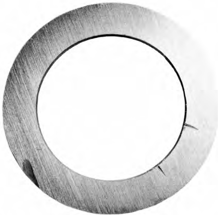
Fig. 26. Pretest Appearance of 2-in., Type 304 Stainless Steel Pipe Specimen, X-1.68 (Test AN-32).
