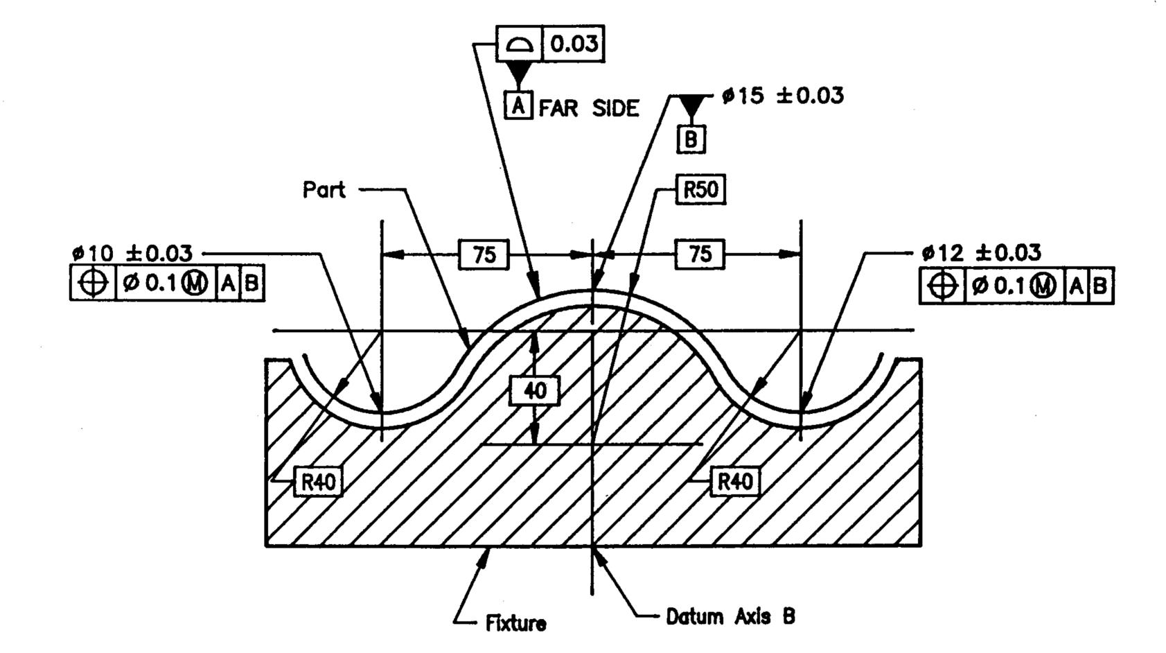
FIGURE 11-17 [Curved Surface as a Datum Feature]
