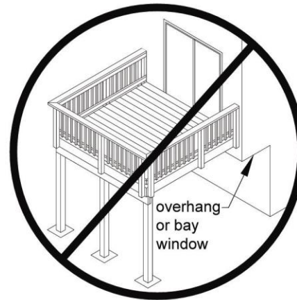
Figure 18. No Attachment to House Overhang with Ledger.
