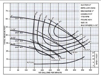
Also, use these correction curves only for centrifugal pumps of conventional design in the normal operating range, with open or closed impellers. Do not use for mixed flow or axial flow pumps. To avoid the effect of cavitation make certain there is ample NPSH.
