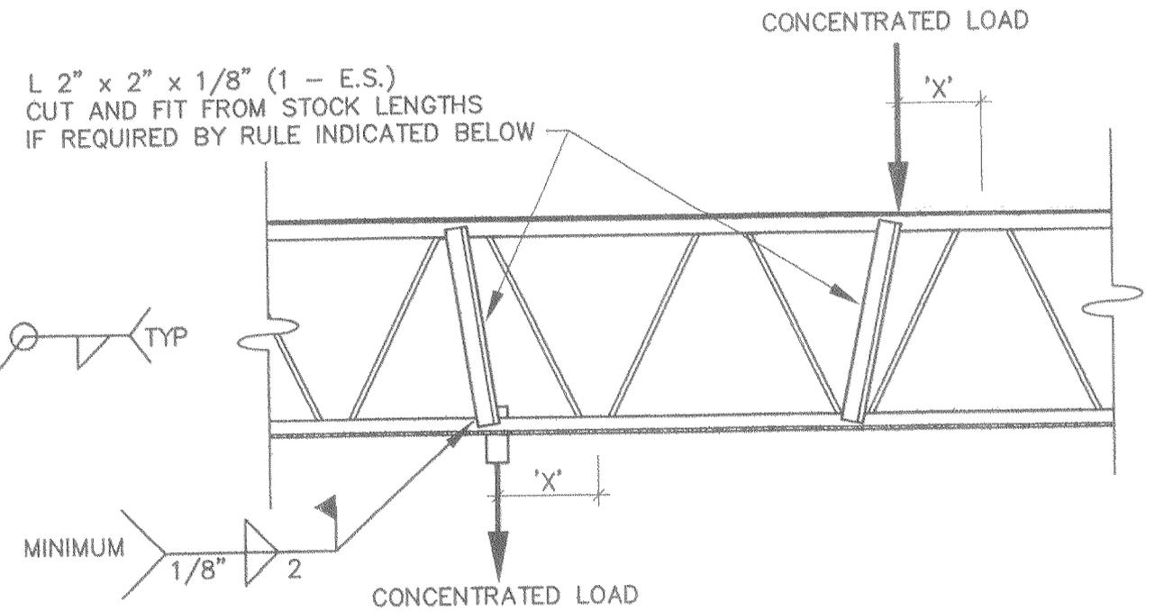
RULE: IF EITHER 'X' IS GREATER THAN TWO INCHES (2") THEN ANGLES SHALL BE ADDED AS INDICATED ABOVE TO TRANSFER CONCENTRATED LOAD TO A PANEL POINT. ALL CONDITIONS SHOULD BE VERIFIED WITH STRUCTURAL ENGINEER.
