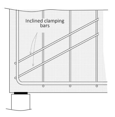
If the bearing length at a support is small and close to the free end of a member, a *sliding shear* failure along a steep inclined crack may occur. Additional small diameter bars may be required perpendicular to the potential failure plane
