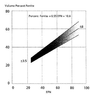
the relationship of EFN to the volume fraction of ferrite measured metallographically. This relationship is shown in Figure 2 and may be expressed as: Volume Percent Ferrite = 0.55 EFN + 10.6
