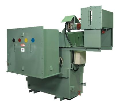
In areas where earth point is not available, a neutral point is created using an earthing transformer. Earthing transformer, having the zig-zag (interstar) winding is used to achieve the required zero phase impendence stage which provides the possibility of neutral earthing condition. In addition an auxiliary windings can also be provided to meet the requirement of an auxiliary power supply.
