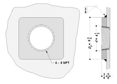
7. By visual estimation the edge ligament indicated above appears to more than adequate for the internal design pressure of 125 lb/in<sup>2</sup>; nevertheless, a check will be made considering it an ultra-short internally threaded projecting nozzle whose minimum thickness will be,
