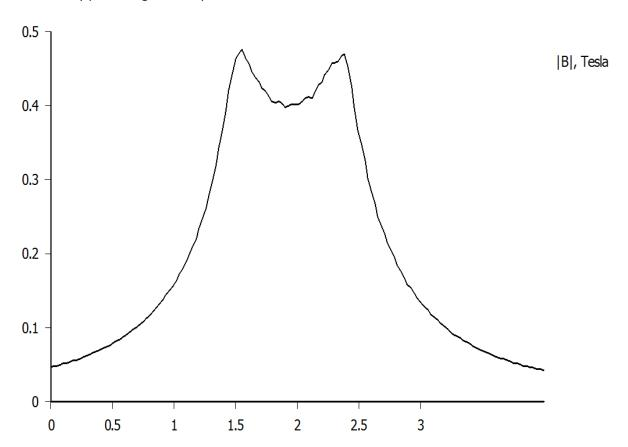
Analysis line 1mm above two 9mm square-section magnets N52 Top faces N next to S
