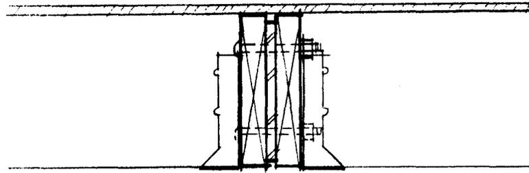
The wood side pieces provide lateral support to the slender steel flitch plate and brace the steel against lateral buckling.
