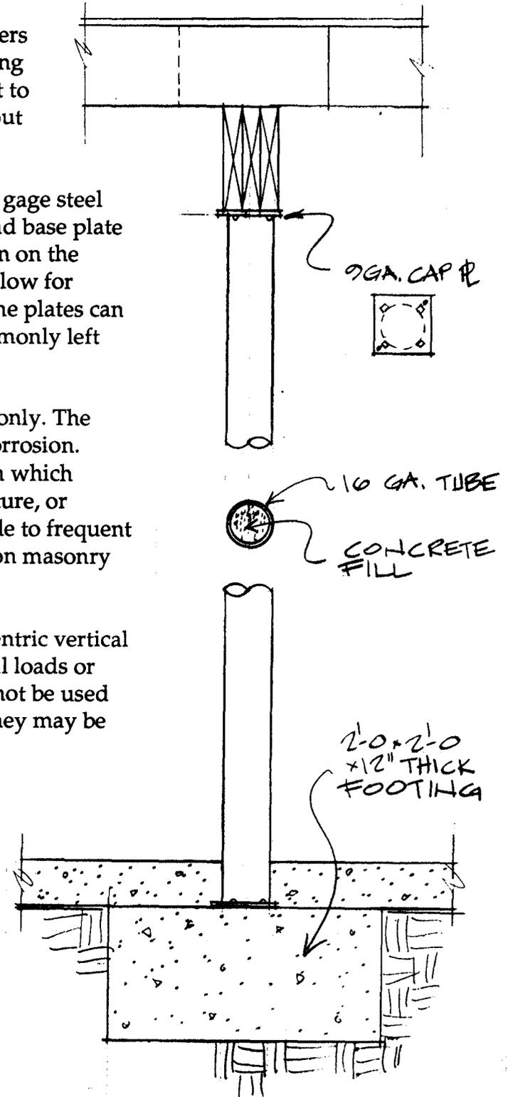
The allowable axial load for structural columns diminishes with increased unbraced length. The load table indicates the allowable column load in kips (1 kip = 1,000 lb.) for various unbraced lengths.
