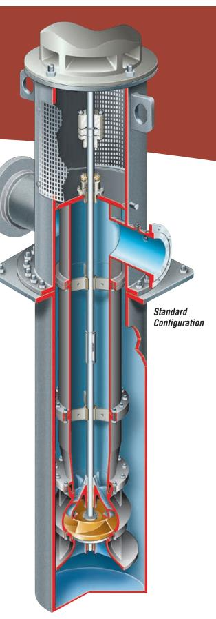
ISO 13709/API 610 (VS6) Vertical Turbine, Double Case Pump
