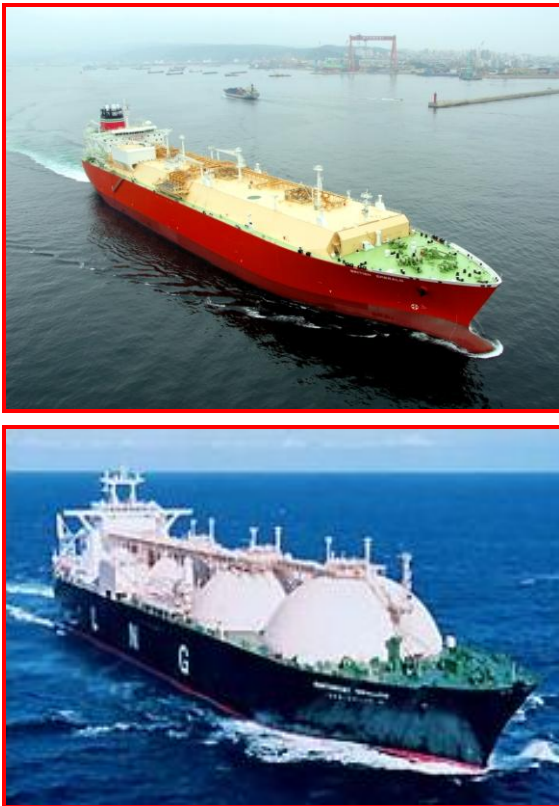
Figure 3. Examples of LNG carrier types: top – membrane design; below – Moss sphere design. (Source: BV 2009)
