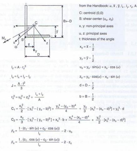
FIGURE 11.7 Definition of cross-section properties.
