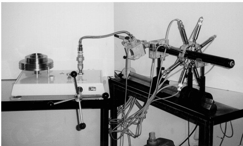
Figure 3: The test rig for investigating the stress-deformation behaviour of HDPE pipe
